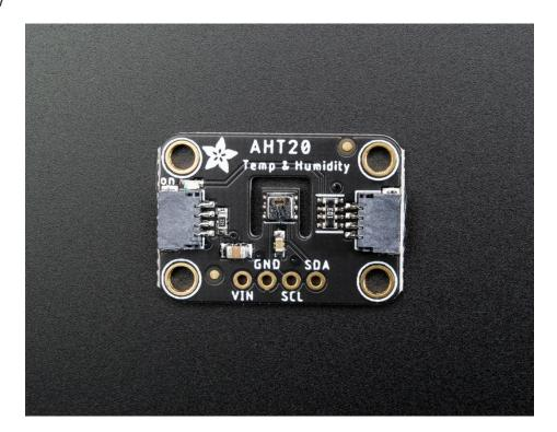
The AHT20 is a nice but inexpensive temperature and humidity sensor<u>from the same folks that brought us the DHT22</u> (https://adafru.it/sb4). You can take sensor readings as often as you like, and it uses standard I2C so its super easy to use with any Arduino or Linux/Raspberry Pi board.
